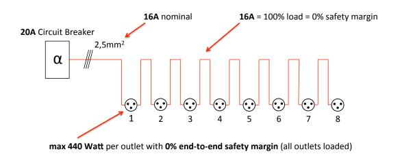
fig 1. Traditional electrical cabling. (220VAC / 16Amp with 8 outlets)
