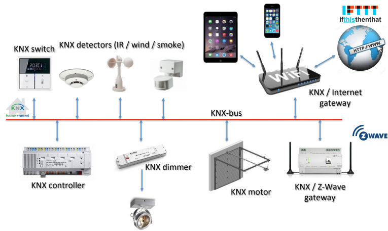
fig 1. Traditional Home Automation example. (i.e. based upon technologies designed with a focus on mass markets, apps, low costs, simple installation ...)
